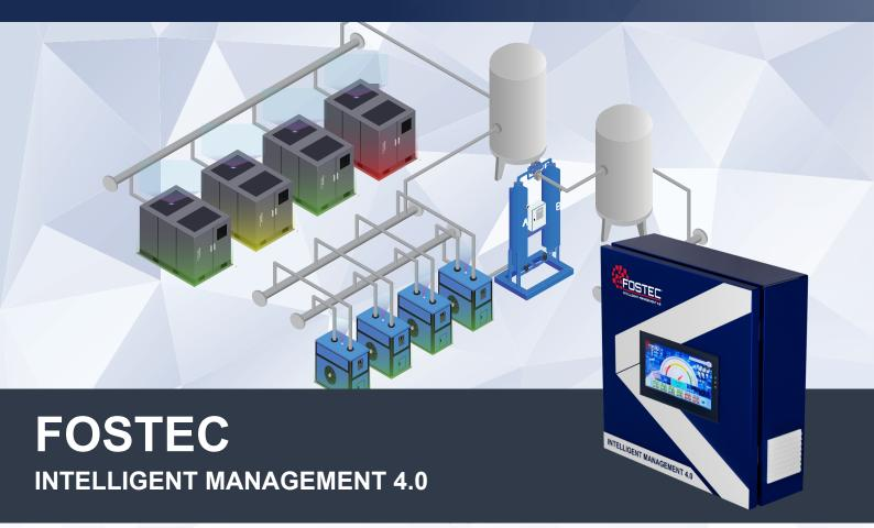
Compressed air is known to be one of the most expensive costs in your production. Multiple air compressors are being used to provide the compressed air to the production line. Most of the time, these Air Compressors are set to run in cascading order with different target pressure on each unit. This causes an unnecessary power consumption to the system.
